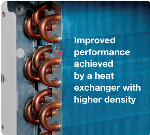
Adopting a slimmer 7.0mm copper pipe. By increasing the number of the copper pipe and fin, the performance level has improved while keeping the heat exchanger size small.
